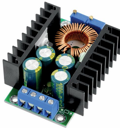
Gambar 2. 13 Modul buck converter berbasis XL4016 [37]
