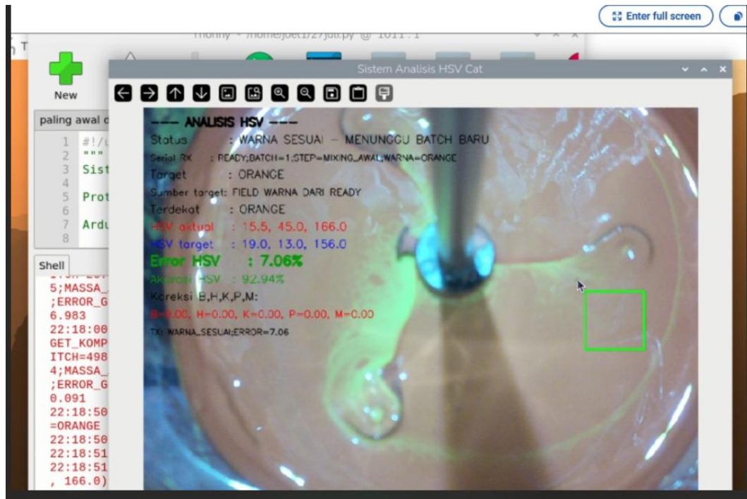
Gambar 4.19 Hasil Proses Mixing Berhasil Tanpa Iterasi
