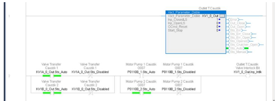
Gambar 3.29 Routine Equipment Rung 1 dan 2
