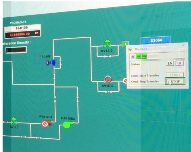
Gambar 4.31 Operator Klik Stop Via SCADA
