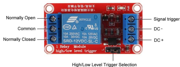
Gambar 2.19 Pinout Relay Optocoupler [24]
