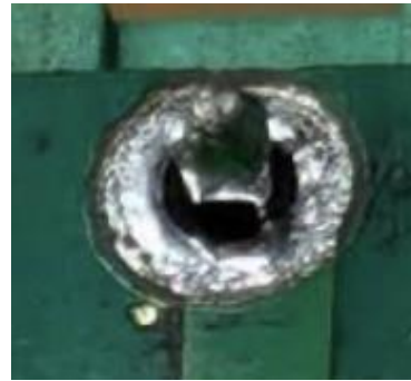
Gambar 2. 4 Cacat Solder Unsoldered[10]
