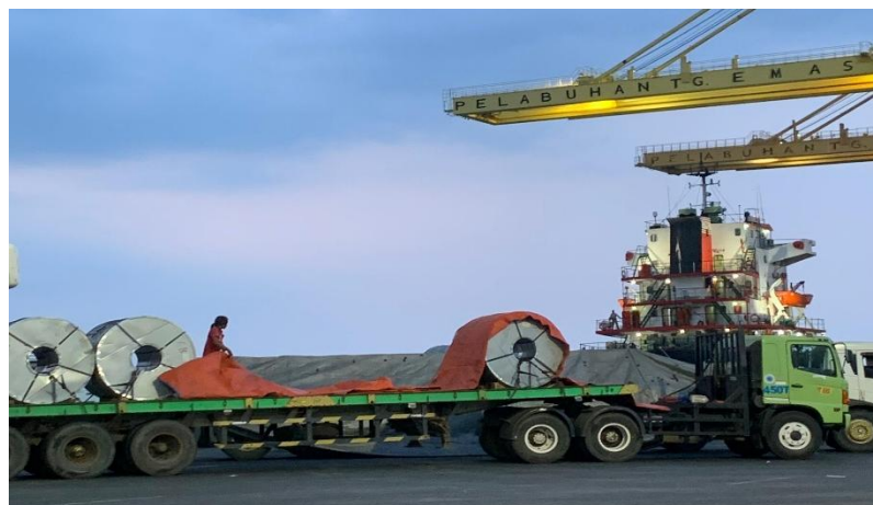
Gambar 4. 8 Proses Peletakan Terpal diatas Muatan Steel Coil
