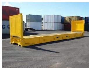
Gambar 2. 4 Flat Rack Container
