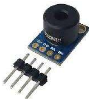
Gambar 2.7 Sensor Suhu Inframerah MLX90614 GY-906 BCC
