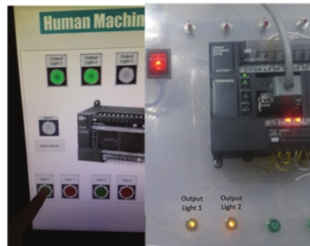
Fig. 3. Discrete inputs testing.
