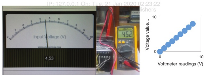
Fig. 6. Analog indicator testing.
