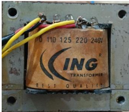
Gambar 2. 22 Transformator Non-CT 5A (Sumber : Pribadi)
