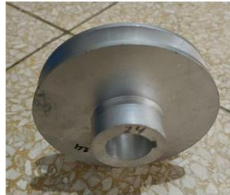
Gambar 2. 25 Pulley Diameter 3 Inch
