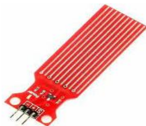
Gambar 2.8 Water Level Sensor
