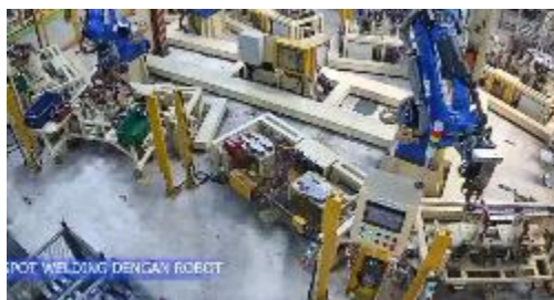
Gambar 3.20 Proses robot spot welding .
