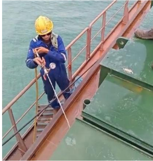
Gambar 2. 16 Hose Test (Sumber : Data milik PT. KTU Shipyard)
