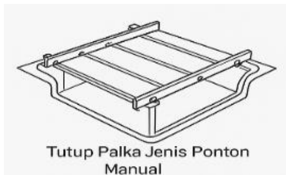
Gambar 2.3 Hatch Cover Ponton Manual
