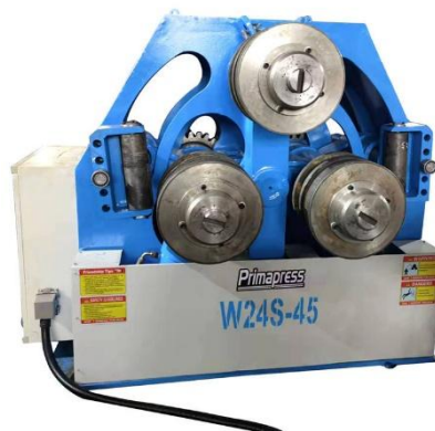
Gambar 2. 2 Mesin Bending Pipa Hidrolik (Sumber: https://share.google/images/Ks11wybG0819UjycD )
