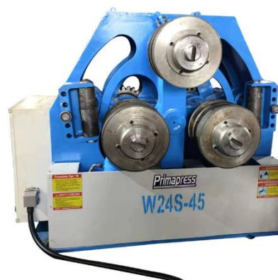
Gambar 2.1.2 Mesin Bending Pipa Hidrolik (Sumber : : https://share.google/images/Ks1IwybGo8i9OlycD )
