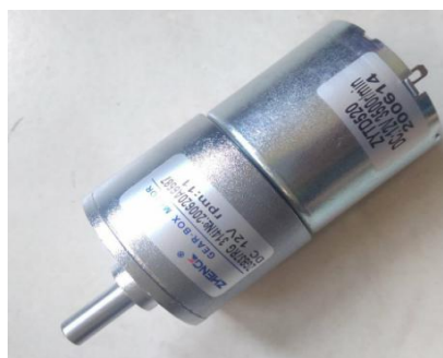
Gambar 2. 12 Motor DC 12 V
