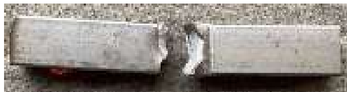
Gambar 4. 7 Patahan stainless steel tampak atas
