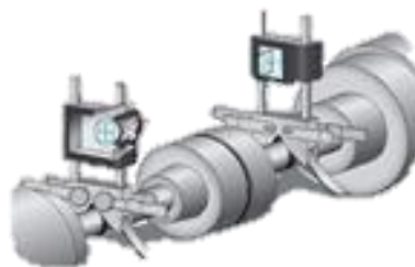
Gambar 2. 16 Shaft alignment metode laser
