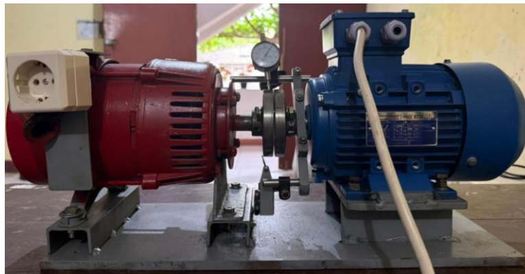
Gambar 4. 1 Hasil fabrikasi simulator shaft alignment
