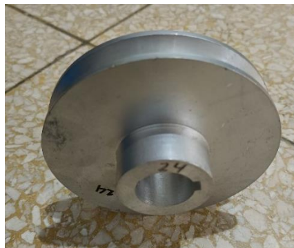
Gambar 2. 14 Pulley Diameter 3 Inch
