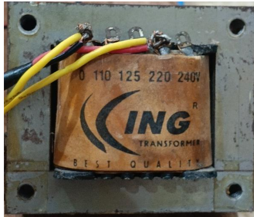
Gambar 2. 11 Transformator Non-CT 5A
