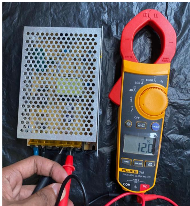
Gambar 4. 2 Pengujian Tegangan Output Power Supply
