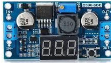
Gambar 2. 10 Lm 2595 Step Down
