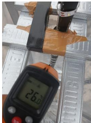
Gambar 5-19 Dokumentasi Pengujian Suhu LED Strip
