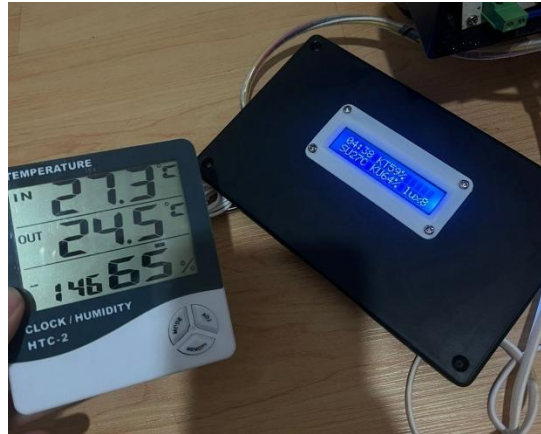
Gambar 4. 7 Kalibrasi Sensor DHT22
