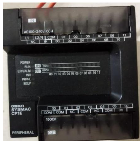
Gambar 2. 8 PLC Omron CP1E
