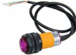
Gambar 2. 16 Sensor proximity infrared
