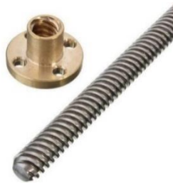
Gambar 2. 31 Lead Screw dan T Nut T8 Lead 8 Pitch 2mm 4Start
