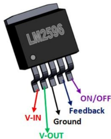
Gambar 2.14 Pinout LM2596
