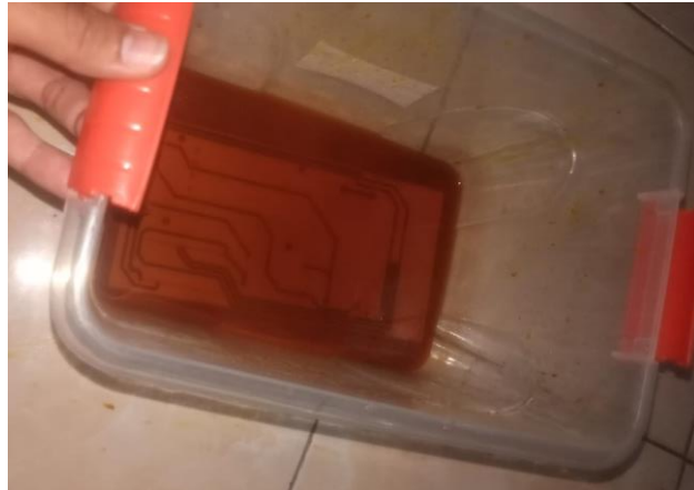
Gambar 4. 9 Proses Etching PCB
