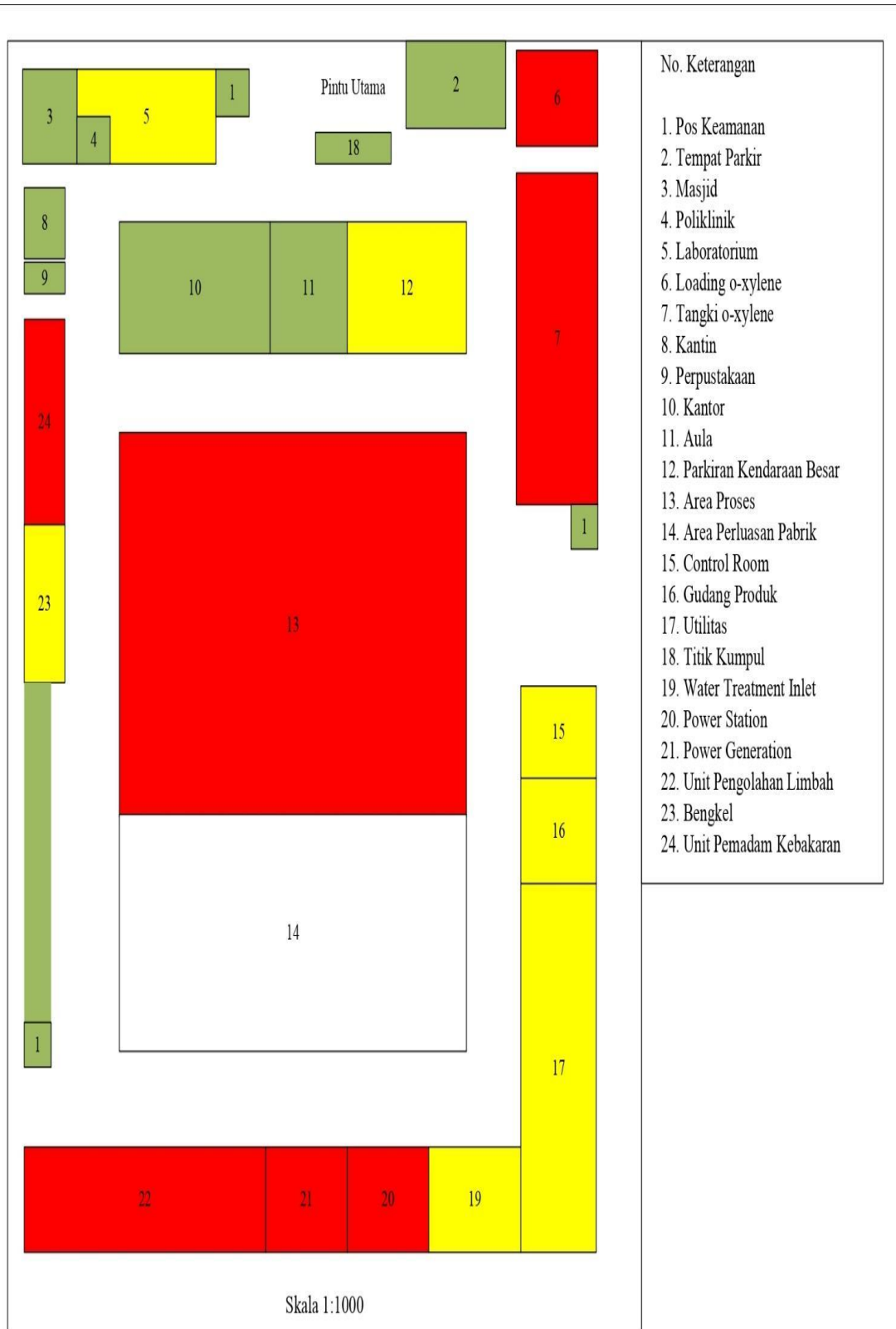
Gambar 2. 1 Layout Pabrik Phthalic Anhydride
