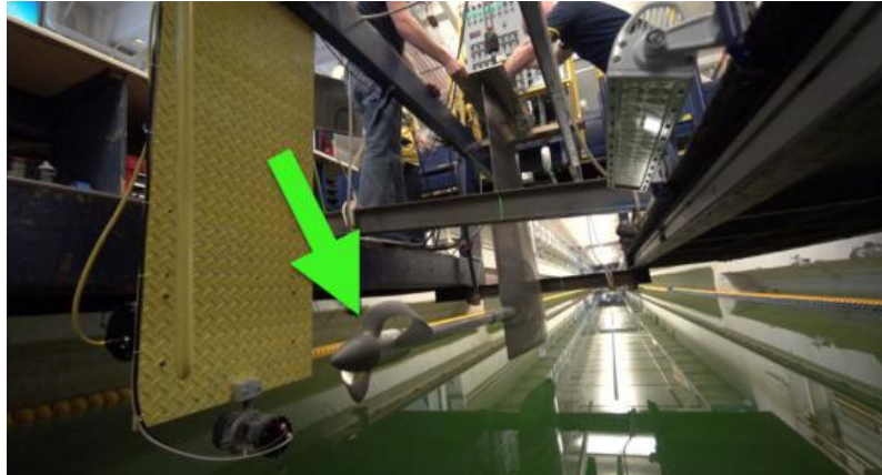
Gambar 2.20 Versi Sharrow Propeller™ Berbilah 2 Dimuat ke Dalam Dinamometer di University Of Michigan's Marine HydroDynamics Laboratory Sumber: University of Michigan's Marine HydroDynamics Laboratory
