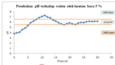
Fig. 6. Graph of changes in pH to time due to the addition of a 5% base solution
