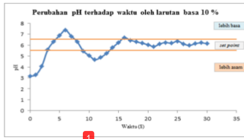
Fig. 7. Graph of changes in pH to time due to the addition of a 10% base solution
