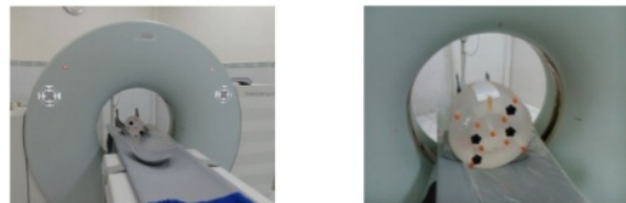
(a) CT Scan (b) Body Phantom PMMA Figure 1. Research instruments
