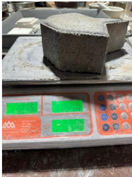
Gambar 3. 30 Penimbangan Paving block
