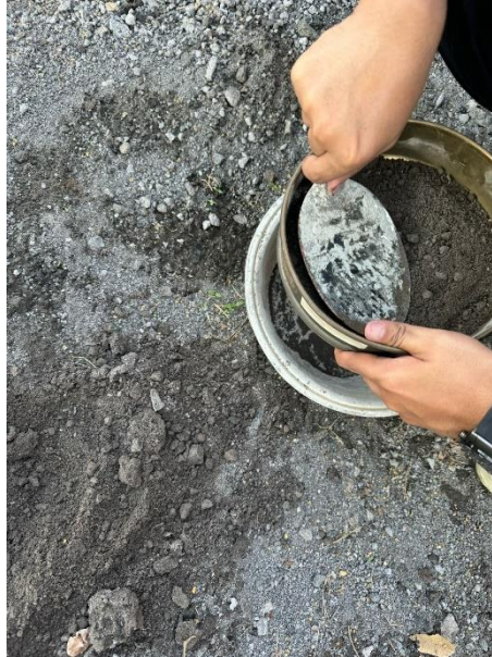
Gambar 3. 11 Pengambilan Sample Pasir Lolos Saringan No. 4
