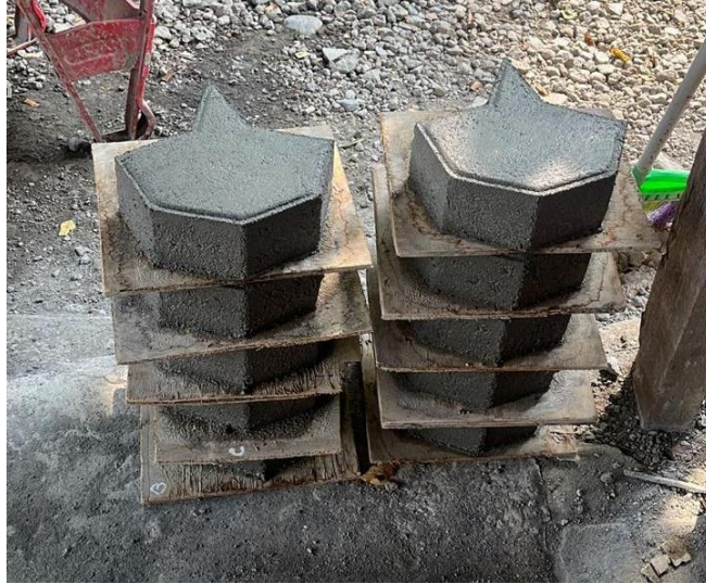
Gambar 3. 20 Persiapan Paving block
