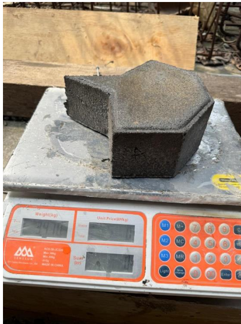
Gambar 3. 29 Penimbangan Paving block Basah
