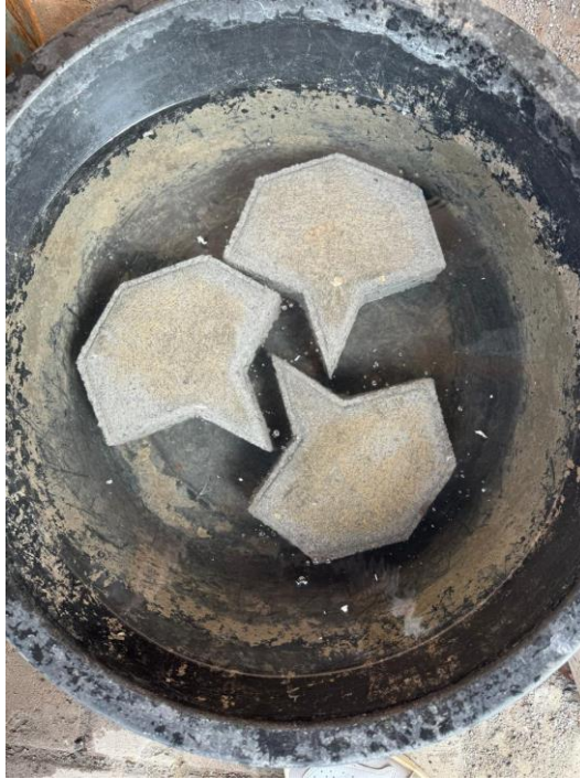
Gambar 3. 28 Perendaman Paving block
