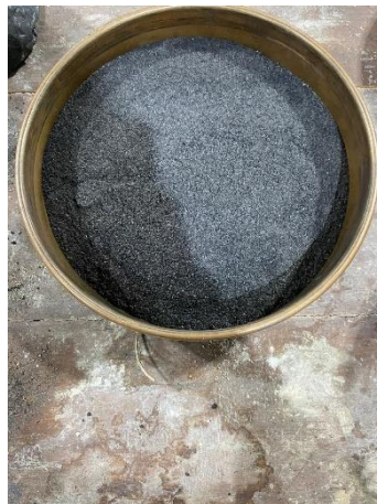
Gambar 3. 19 Abu Boiler Kelapa Sawit
