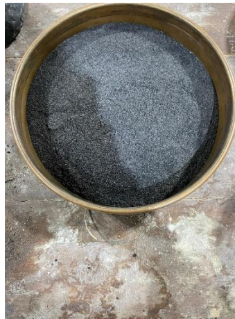
Gambar 2. 1 Abu Boiler Kelapa Sawit
