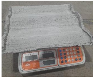
Gambar 3. 60 Penimbangan genteng beton kering
