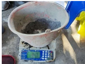
Gambar 3. 27 Menimbang Masing-Masing Bahan Material Paving Block
