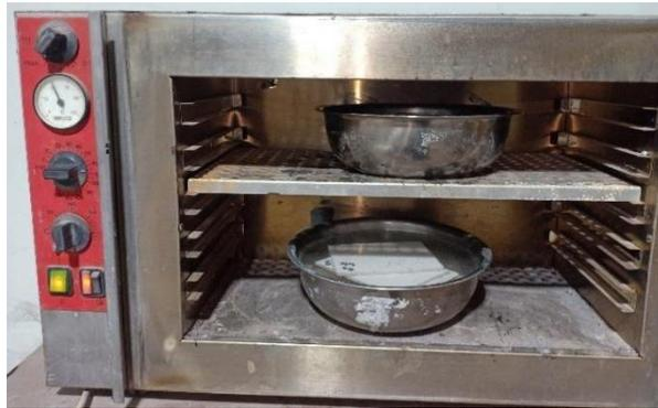
Gambar 3. 27 Perendaman Benda Uji didalam Oven
