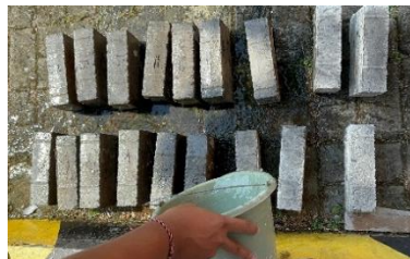
Gambar 3. 58 Curing paving block
