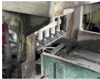
Gambar 3. 54 Proses perataan permukaan benda uji paving block
