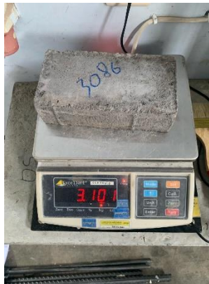
Gambar 3. 43 Proses penimbangan berat basah paving block
