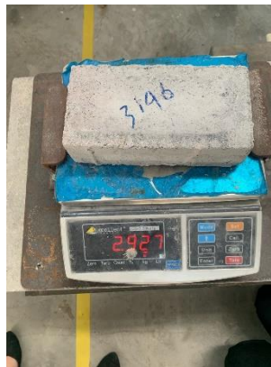
Gambar 3. 45 Penimbangan berat kering paving block
