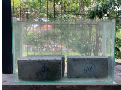
Gambar 3. 42 Proses perendaman paving block
