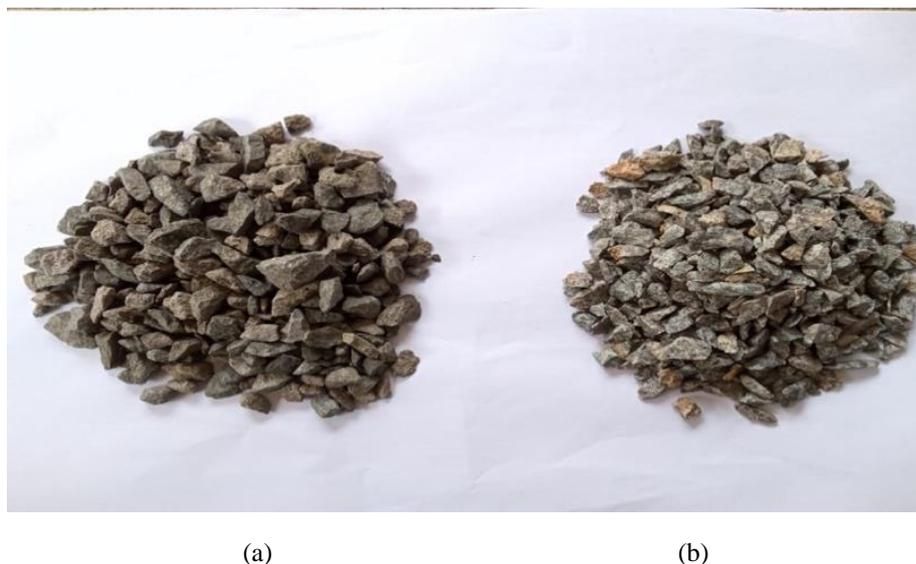
Gambar 3.2 (a) Agregat Andesit, (b) Agregat Diorit
