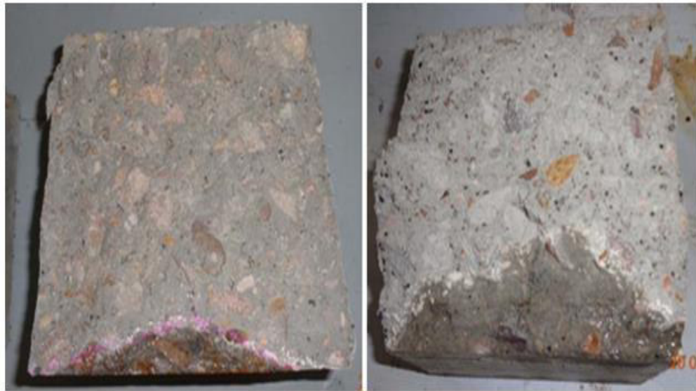
Gambar 2.21. Pengukuran kedalaman penetrasi air ( Measurement of depth of water penetration, Gupta et al, 2017 )
