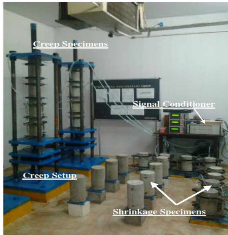
Gambar 2.14. Pengujian susut dan rangkai ( Test setup of shrinkage and creep specimens ) (Gedam, et al, 2016)
