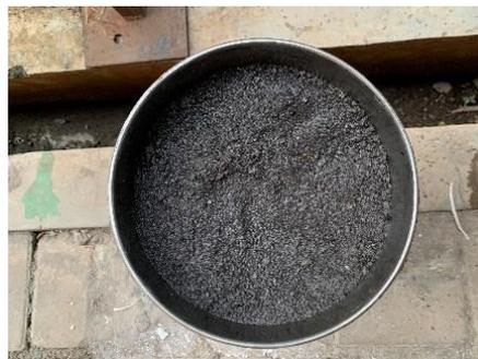
**Gambar 3.9** Pencucian Material Lolos No.200 Agregat Halus
