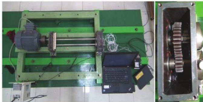
FIGURE 1. Data acquisition process of vibration signal
