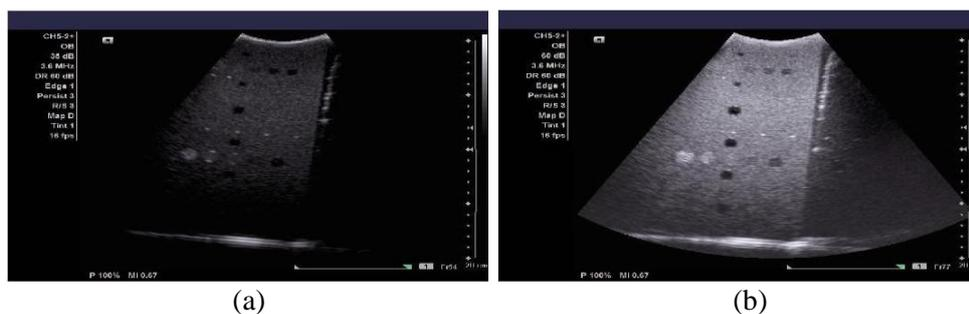
**Figure 1.** Scanned phantom image using 3,6 MHz Frequency with gain variation of (a) 30 dB and (b) 60 dB.
