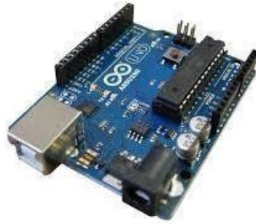
Gambar 2.1 Atmega328 board Arduino Uno (Widyastuti dan Ishafit, 2019).
