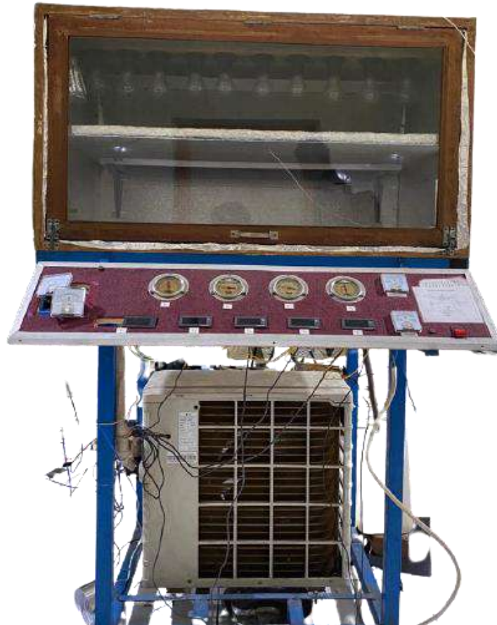
Gambar 3.2 Test Bed Air Conditioner
