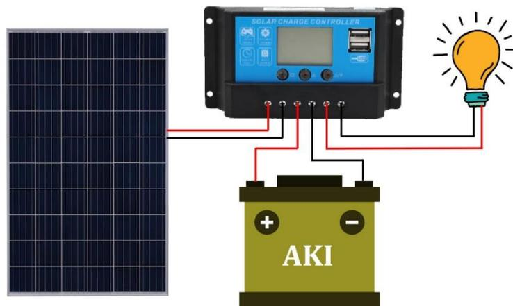
**Gambar 4.7** Wiring *Solar charge controller* Pada Kondisi Saklar ON
