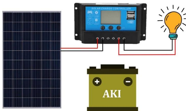
**Gambar 4.6** Wiring *Solar Charge Controller* Pada Kondisi Saklar OFF
