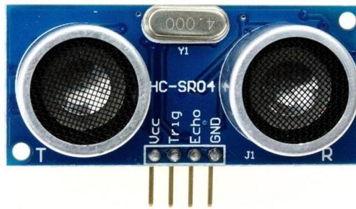
Gambar 2.4 Sensor Ultrasonic HC-SR04
