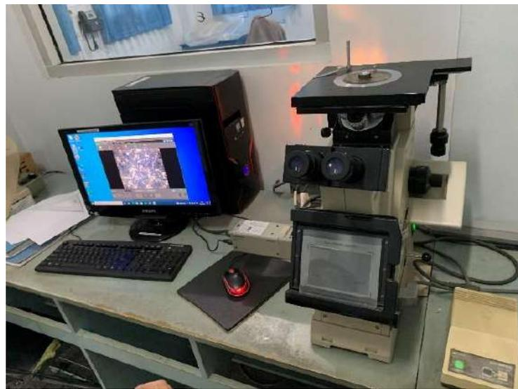
Gambar 3. 3 Metallurgical Microscope
