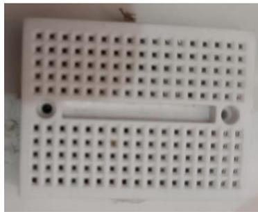
**Gambar 3. 21 Papan Breadboard**
