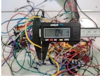
**Gambar 3. 20 Diameter Kabel AWG 26**
